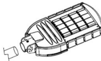
2. Adjust the led street lights to a suitable position according to your requirements for lighting. Then tight the screws. The mounting bracket is adjustable each 5 deg from  $-15$  deg to  $15$  deg , 90 deg for straight pole is available.
